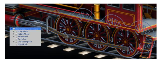
These rods are attached to each other and to the locomotive wheels by Unity default Position Constraint and Look At Constraint components. These constraints makes sure the rods will move accordingly to the wheels rotation.
