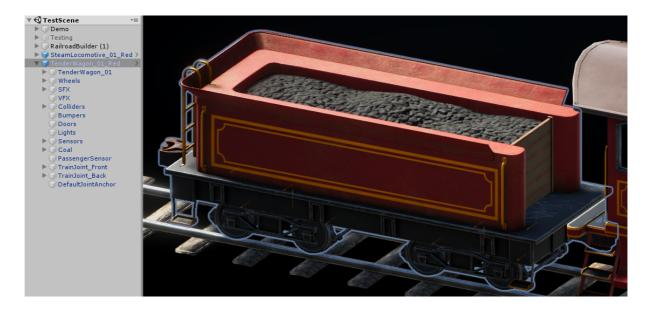
The tender wagon coal is a separated model, so it can be disabled, removed or replaced by a custom model.
